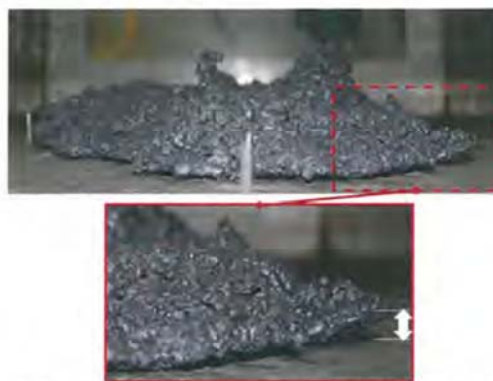
Figure 40: The melt spread in PULiMS-E1 experiment (side view). The volatile particle debris have been removed while solidified core of the melt remained intact.
