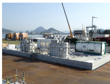
Detoxification of large-scale transformers through heat treatment
