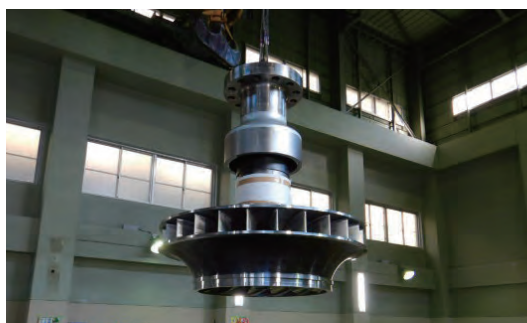
Highly efficient runner at Hirono Hydro Power Station (Naka-cho, Naka-gun, Tokushima Prefecture)
