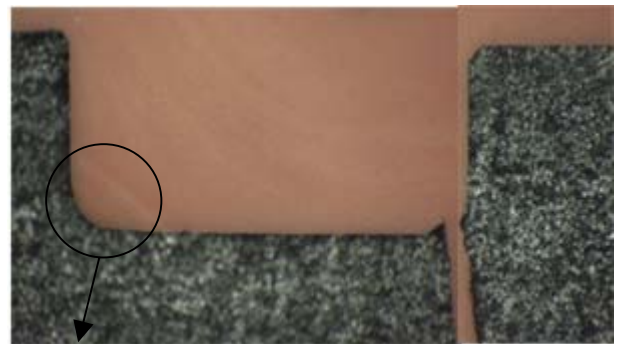
曲率半径 R:0.81mm R 止まり:0.40mm 継手側:135°
